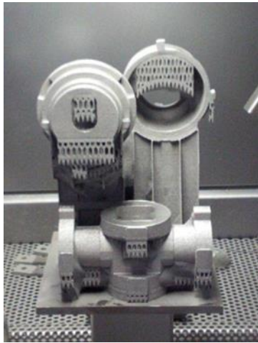
Antenna Pedestal Arms for Radar system
