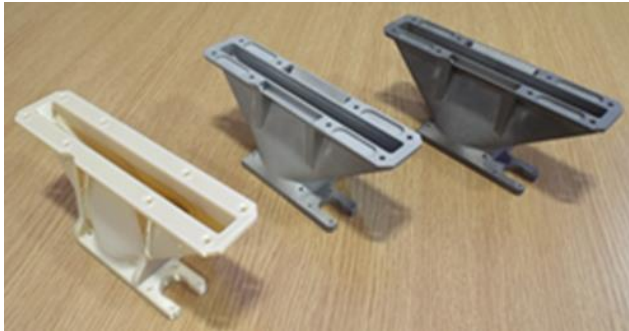
Microwave waveguides for Radar system
