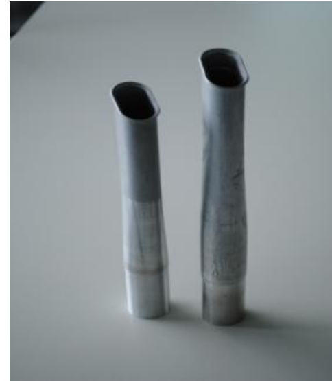
Ducts for M346 trainer
