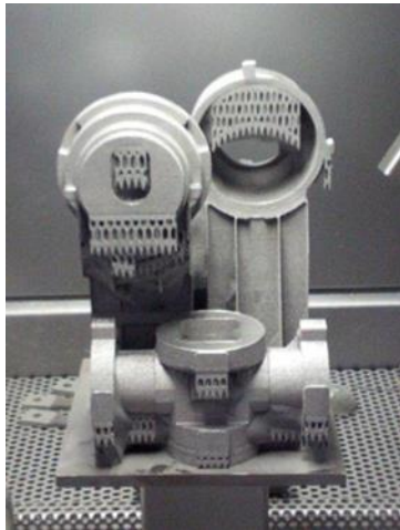
Antenna Pedestal Arms for Radar system
